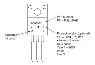
Example: This is a xxxxxxxFP with assembly lot code AC, assembled on WW 19, 2001 in the assembly line "X"
